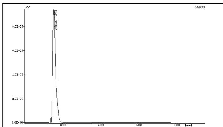
**Fig. 3: The chromatogram represents the pure bulk drug of Orlistat**
