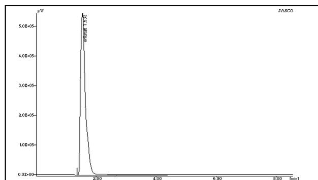
**Fig. 5: The chromatogram represent peak of orlistat in formulation 2 (Lipocut capsule).**
