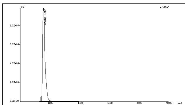
**Fig. 4: The chromatogram represents the Orlistat formulation1 (Zerofat).**
