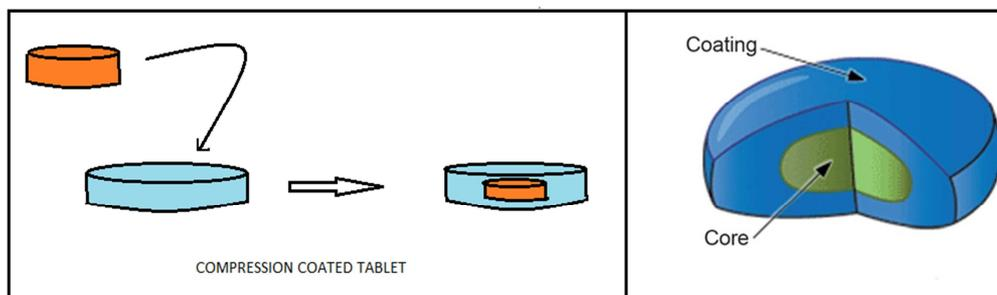
Figure 7: Preparation of compression coated tablet
