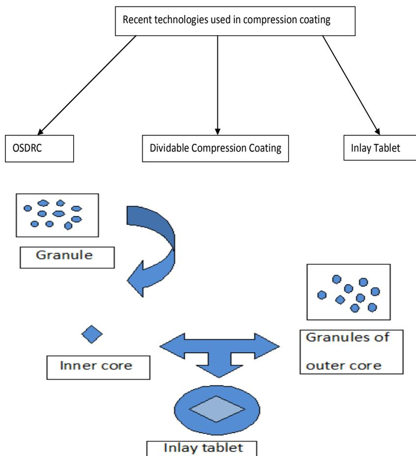
**Figure 2: Preparation of Inlay tablet**
